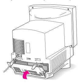
**WARNING** Never turn on your computer unless all of its internal and external parts are in place. Operating the computer when it is open or missing parts can be dangerous, and can damage your computer.
